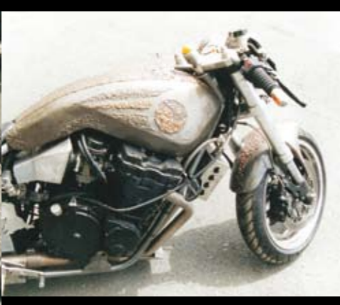
Funky Suzuki had swarf from different coloured metals set in resin to create graphics and a YinYang on the tank. Far out man.
